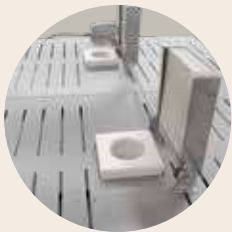
Manual and motorized exhaust air opening in the roof for faster cooling. Operating lever on the right-hand side of the furnace (above the switchgear).
