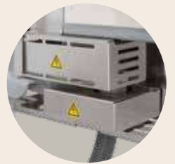
Protected door contact switch
