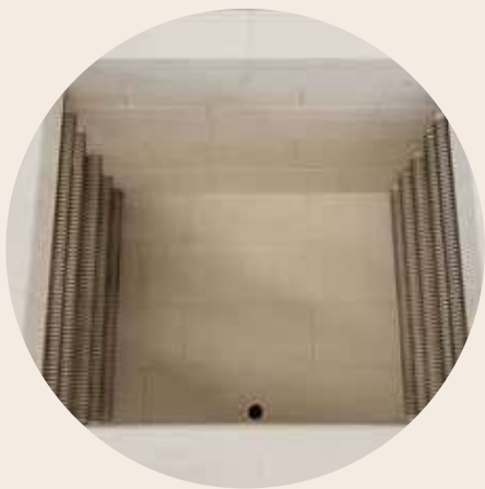
Heating elements on support tubes on both sides ensure free heat radiation
