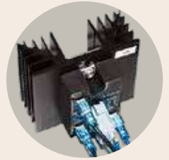
Low noise electronic relays
